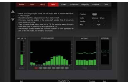
The next step will allow you to set up the level of your speakers. The ideal situation is to have the Ovation at Fader 7 and adjust the amp levels for the proper gain (\*) At this step and at fader 7.0, the screen channels should be at 65dBC and the subwoofer at 80dBC. This is also a good time to balance the High and Low for bi amp systems. High, Low and Mid for triamp etc.
