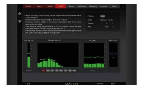
Here is the HF and LF together relatively balanced and at 65dB
