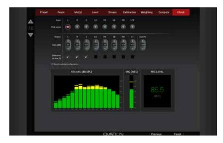
The Check step allows you to verify and adjust SPL if necessary. The Optimizer will set the screen channels at 85dB and surrounds at 82dB (-3dB on the settings). Subwoofer(s) will be between 87-90 dB. It is also possible to monitor the output channels on Aux1/Aux2 and setup the associated volume.
