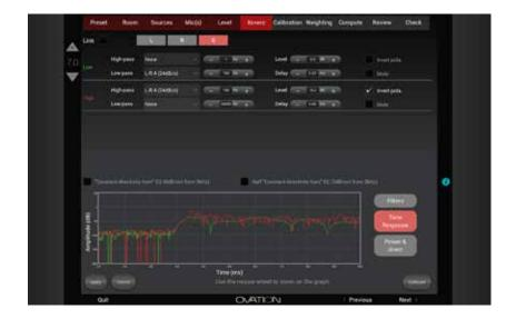
Here we see the Power and Direct response. With perfect timing, you will see the least amount of dip in the frequency response. There is a possibility to fine tune this Time using Power and Direct graphs to guide you. This is covered in an advanced document. Link here\*.
